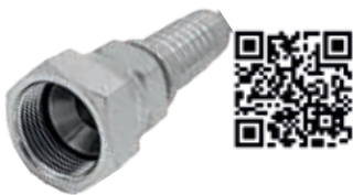
BSP JIS GAS FEMALE 60° CONE SEAT JIS B8363 (JAPONESA)
